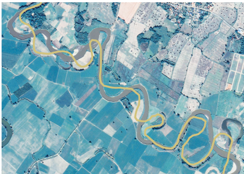
Figure 4.5 A section of the Myanmar-Thailand boundary along the Ruak river. The boundary has been demarcated along the course of the Ruak as it was mapped in the 1940s, and the boundary does not move with the river. As a result, numerous pockets of territory are now located on the 'wrong' side of the river and are difficult for local farmers to access. The field patterns in the image suggest that the practical consequence is that farmers continue to treat the river as the boundary, with farmers from Myanmar cultivating land that is officially part of Thailand and vice versa. Image: Google, CNES/Airbus.
